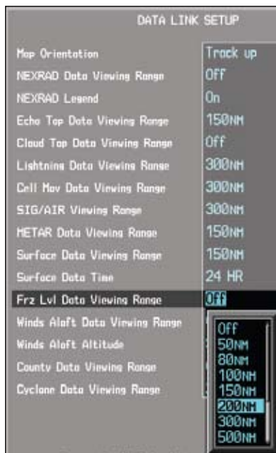
Figure 4-60 Freezing Level Viewing Range Selection
